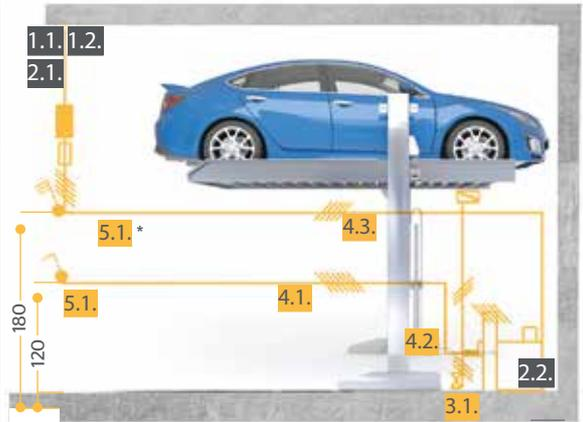
\*Option: The height of the floor stand for key switch is 180 cm.
