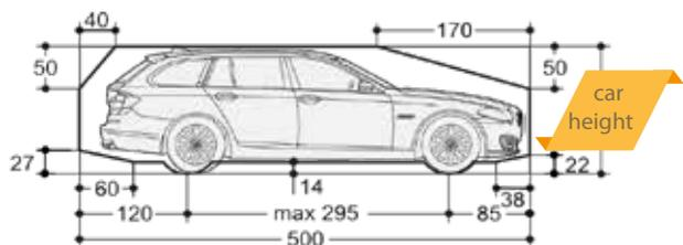
The "car height" including roof rails, antenna and others must not exceed the mentioned max car height dimension.
