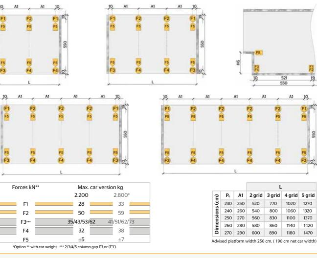
Systems are fixed by heavy duty anchor bolts with a drilling depth of approx. 14 cm.
